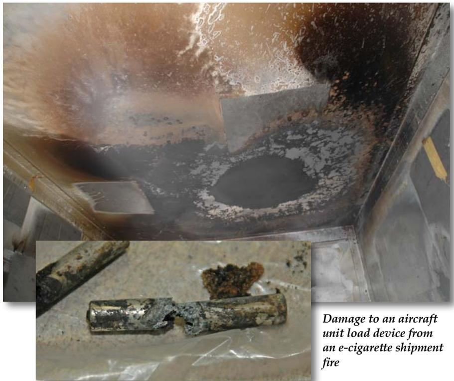
*Damage to an aircraft unit load device from an e-cigarette shipment fire*
