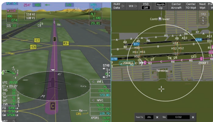
TaxiWiz can provide a pilot with a taxi waypoint path on the 2-D and 3-D airport map. Currently this path is entered via scratchpad entry and/or graphical selection.
