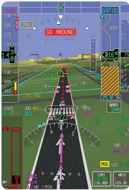
The current energy state of aircraft prediction (as calculated by threshold crossing height and speed with manufacturer-provided performance data) indicates there is insufficient runway length available to make a safe landing. ROAAS provides an aural and visual display “Go Around.”
