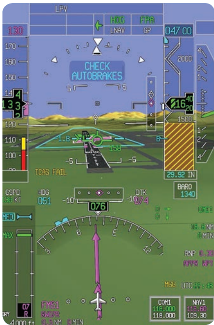
Current autobrake setting (medium) is predicted to not stop the aircraft on the available runway landing surface. ROAAS provides a visual “Check Autobrakes.”
