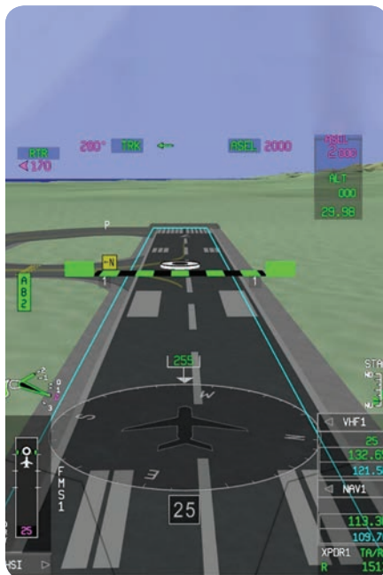
After landing, the display transitions to an exocentric mode. The ROAAS white deceleration “donut” indicates current braking performance (which is just past the Max Brake Green line). The donut may be used in conjunction with the 3-D airport map to plan the runway exit.
