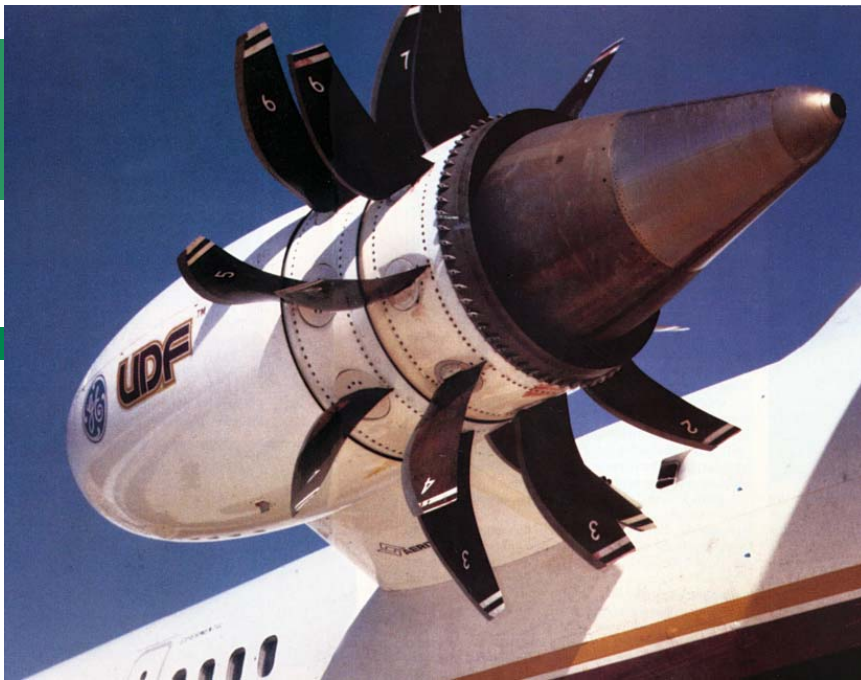
ABOVE: GE's Unducted Fan (UDF) demonstrator in 1988. LEFT: Rolls-Royce open-rotor concept. ABOVE RIGHT: General Electric's GenX, successor to the CF6, will power the B-787 and B-747-8. BELOW: CFM's LEAP 56 composite engine will have a fan diameter of 14 feet.
